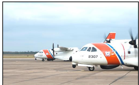
Two Coast Guard HC-144A Ocean Sentry Maritime Patrol Aircraft, the replacement for the HU-25 Falcon. The aircraft have the size, range and reconfiguration capability to enable the execution of multiple Coast Guard missions.
