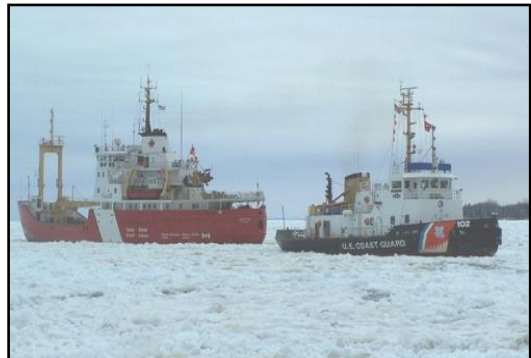
Canadian Coast Guard icebreaker GRIFTON and U.S. Coast Guard Cutter BRISTOL BAY, a 140-ft Ice Breaking Tug, work to flush the ice jam in the St. Clair River March 21, 2010, as part of Operation COAL SHOVEL. Waterborne cargo and associated activities contribute more than $649 billion annually to the U.S. Gross Domestic Product.
