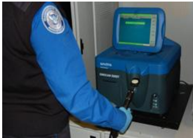
A Transportation Security Officer using Electronic Trace Detection technology to test for explosives on an aviation passenger's carry-on luggage
